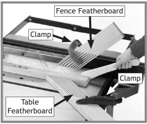
**Figure 67.** Example photo of featherboards mounted with clamps.
